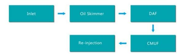
The oil contained wastewater firstly passes through the CPI unit to remove slick oil; then in the DAF unit emulsified oil will be largely reduced; finally through the CMUF unit, most of SS and oil content of wastewater will be
